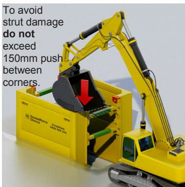
3. Push down on each corner of the box sequentially, but not more than 150mm increments, until formation achieved
