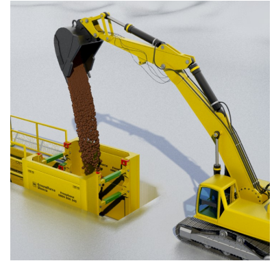
6. Begin to backfill and compact in stages.
