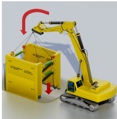
2. Lower the assembled box into the guide trench.
