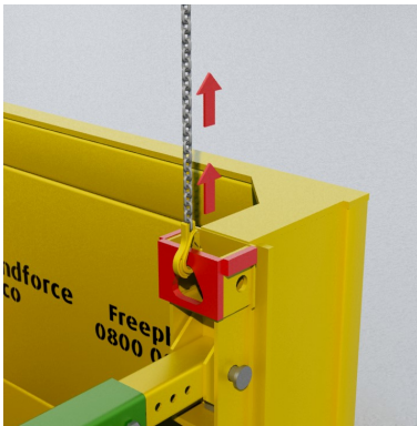
7. Using a single heavy duty chain, attach to each corner of the box and lift by no more than 150mm each time. Do not snatch the chain
